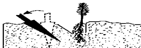
4. Pull dibble back to close bottom of tree planting hole.
