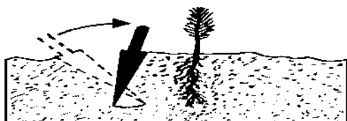
5. Push dibble forward to close top of tree planting hole.
