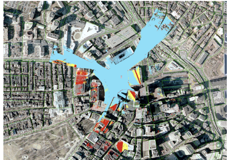
Figure 4. Signal-to-interference analysis with red indicating significant interference.
