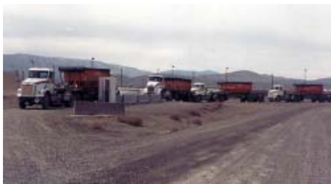
Trucks carrying contaminated material pass through a weigh station enroute to the Environmental Restoration Disposal Facility. The daily average is 150 truckloads totaling 3,000 tons.
