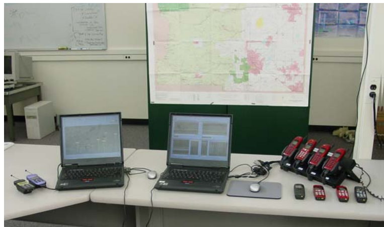
CDMA and multi-technology drive test systems.
