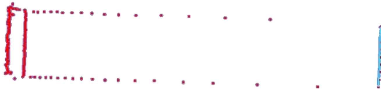
Figure 16: The detected front wall of the truck is shown in cyan color on the right. Depth of the truck measured 16.45 m from the forktruck AGV. Note the truck door was partially detected as an overhanging object.
