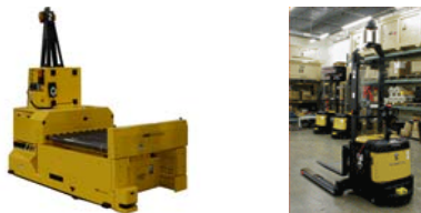
Figure 1 – Typical AGVs used in the material handling industry: unit load (left), forklift (right)
