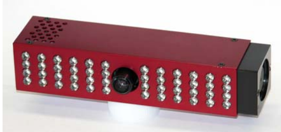
Figure 1 - CSEM SwissRanger-2 3D Range Camera. The camera simultaneously generates intensity images and range information of targets in its field-of view at a rate of 20 Hz with an active range of 7.5 m.
