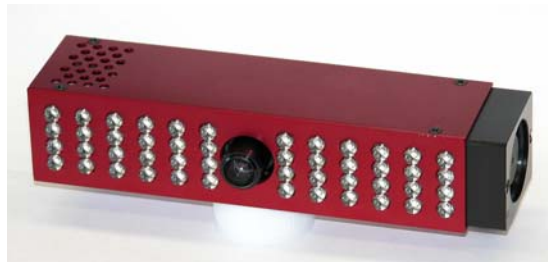
Figure 1 - The TOF 3D range image camera. The camera simultaneously generates intensity images and range information of targets in its field-of view at a rate of 20 Hz with an active range of 7.5 m.
