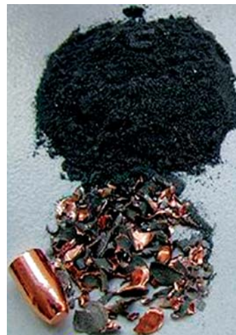
Figure 1: Frangible 9 mm bullet and remains after impact.
