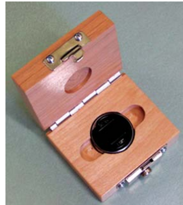
Figure 1: Prototype of new steel microhardness SRM.
