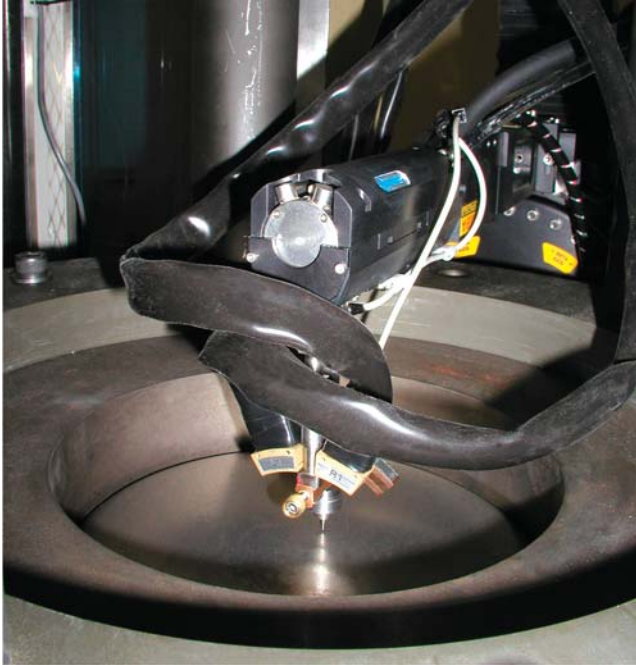
Figure 2: Newly installed X-ray stress measuring system as it takes data on sheet metal being deformed in biaxial tension.
