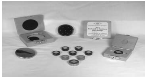
Figure 1. SRM test blocks for Rockwell hardness and Vickers and Knoop microhardness
