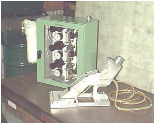
Figure 4. Fluidized feedshoe and associated equipment for improving the flowability of fine or irregularly shaped powders into die cavities.
