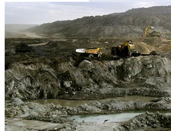
Open-pit mining uses shovels and large trucks to remove oil sand — a thick and sticky form of crude oil — in Fort McMurray, Canada. (Photo by Melina Mara/The Washington Post , reproduced with permission.)
