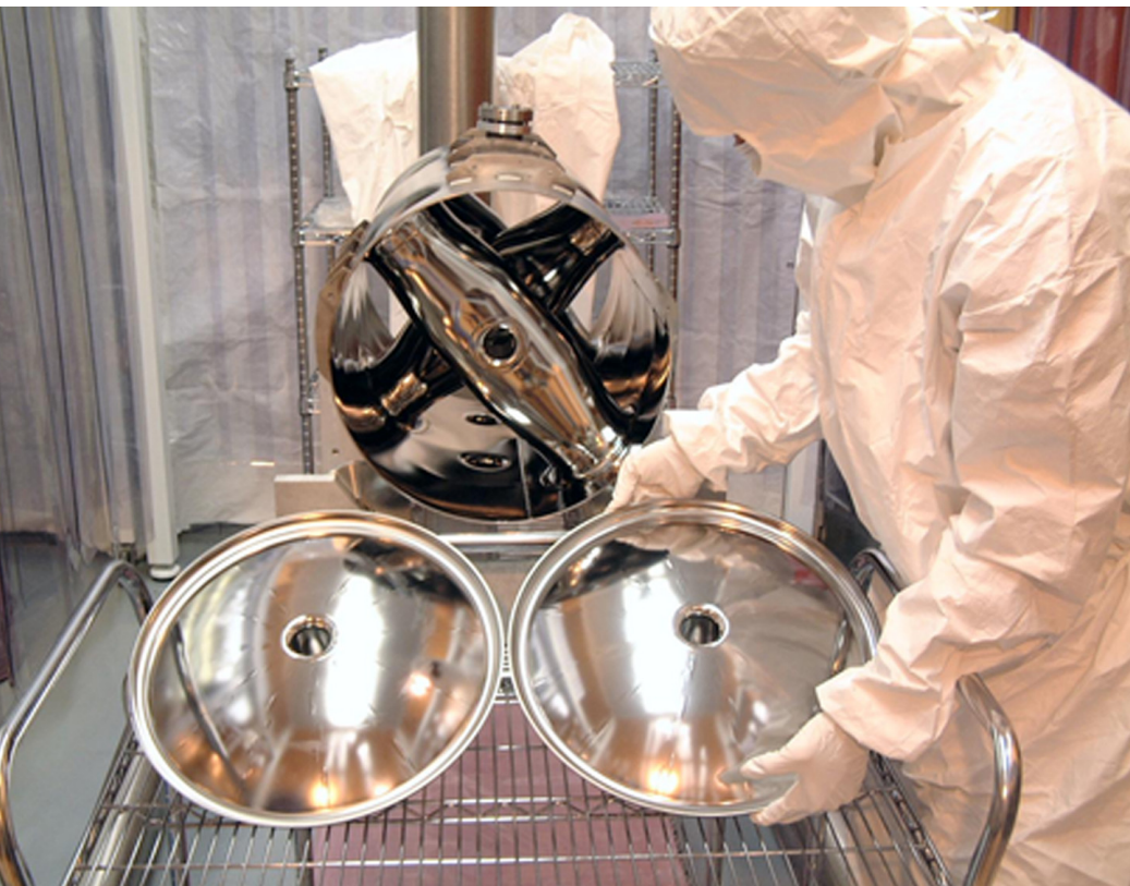
A superconducting triple-spoke cavity is prepared for electropolishing in a clean room.
