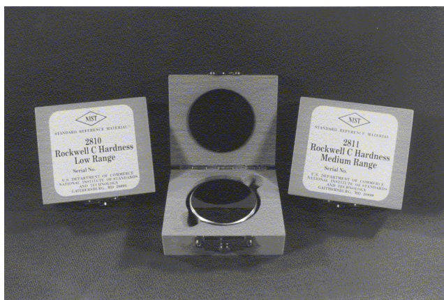
Rockwell hardness SRMs for the HRC scale.
