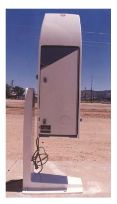
The Ceilometer is located near the back of the instrument van. The Ceilometer measures the distance from the ground to the bottom of a cloud directly overhead. This distance is called "cloud base height." The Ceilometer can measure cloud bases up to about 8 kilometers above the surface. The Ceilometer sends out a pulse (flash) of light and measures how long it takes for it to come back to the Ceilometer after being reflected off the bottom of a cloud.
