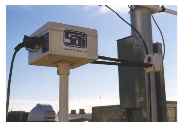
The ORG is mounted on a small pole near the meteorological tower. The ORG measures the rate of rainfall in millimeters per hour (mm/hr). The ORG sends a beam of light (which you cannot see) from one of its ends to a detector at the other end. When raindrops fall, they break the beam. The rain rate is measured by the ORG by measuring how often the beam is broken. The rain rate can be used to calculate the total amount of rain that has fallen in any given period.
