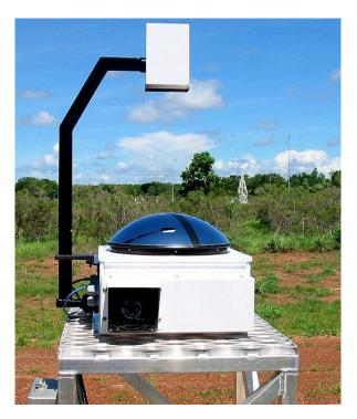
The Total Sky Imager (TSI) provides time series of hemispheric sky images during daylight hours, and retrievals of fractional sky cover for periods when the solar elevation is greater than 5 to 10 degrees.
