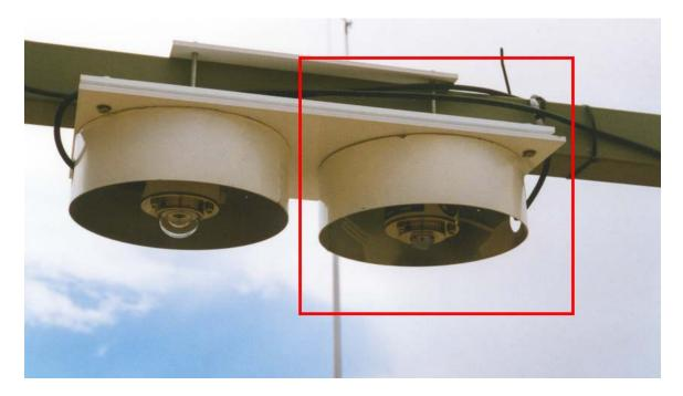
The PIR measures the amount of infrared (heat) energy that falls on a sensor under the shiny dome. This energy is the same heat energy you feel when standing next to a campfire or cook stove. The shiny dome reflects solar radiation but allows infrared radiation to pass through.
