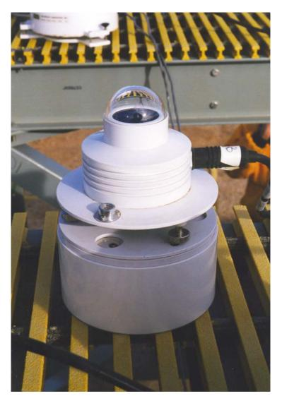
The instrument mounted on the SKY stand, measures ultraviolet radiation. This component of radiation may cause skin cancer. The amount of this radiation that reaches the surface of the earth depends on the amount of ozone in the upper atmosphere.
