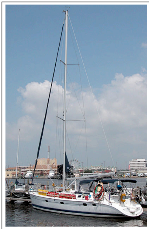
Figure 4.2.5. The Summer Breeze , a 46' sloop, served as the research vessel for the 2005 MPS cruise. To extend the reach of the vessel, 34 red and yellow jerry cans were lashed to the deck. One of the towed hydrophones can be seen coiled up at the port stern. (Photo: Bill Lang)
