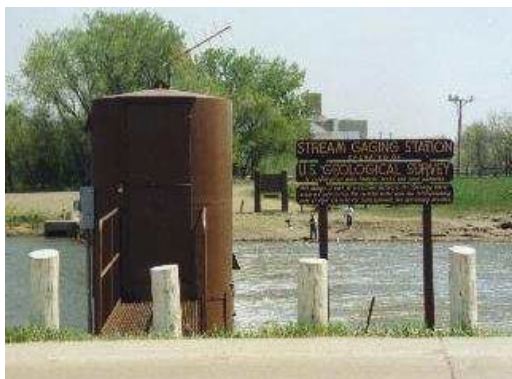
U.S Geological Survey gaging station with satellite antenna.
