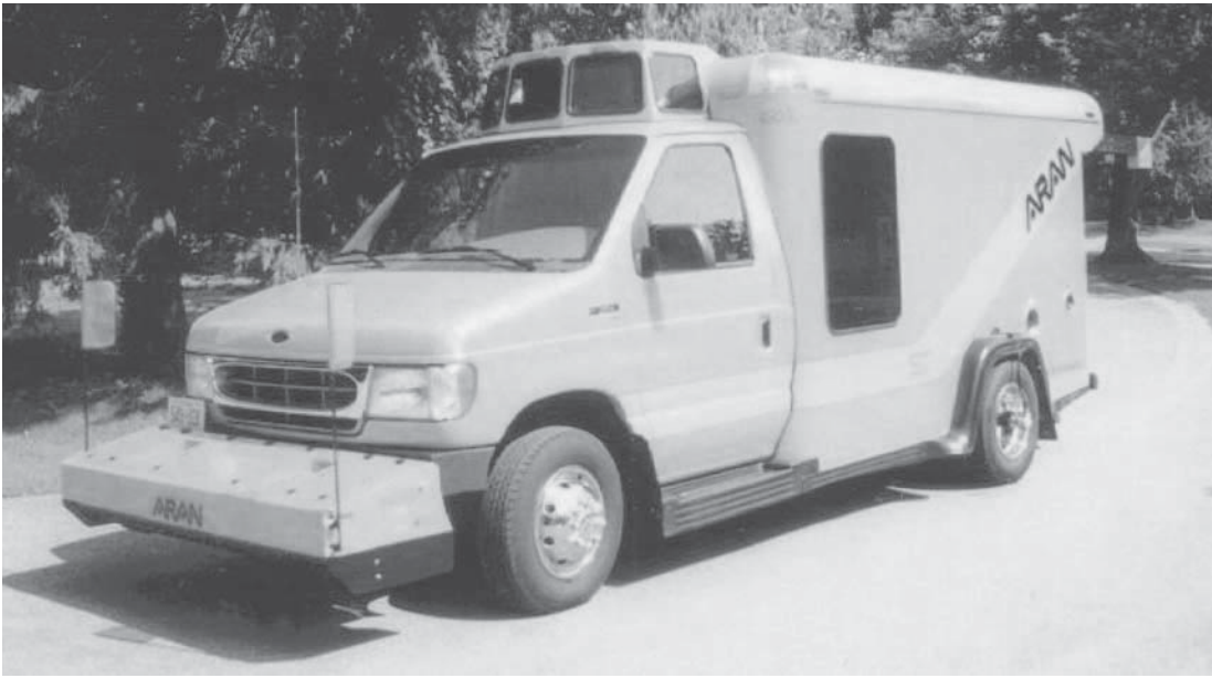
Automated Road Analyzer vehicle is equipped with state-of-the-art technology that enables FHWA staff to collect pavement data on the roadway network within the National Park System.
