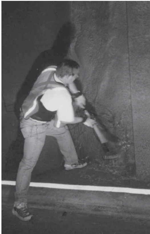
Investigator uses a title hammer to survey seismic characteristics of Zion–Mt. Carmel Tunnel.
