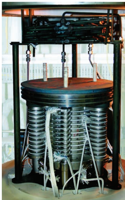
A prototype of the first fuel cell to pass the initial SECA technology hurdle.
