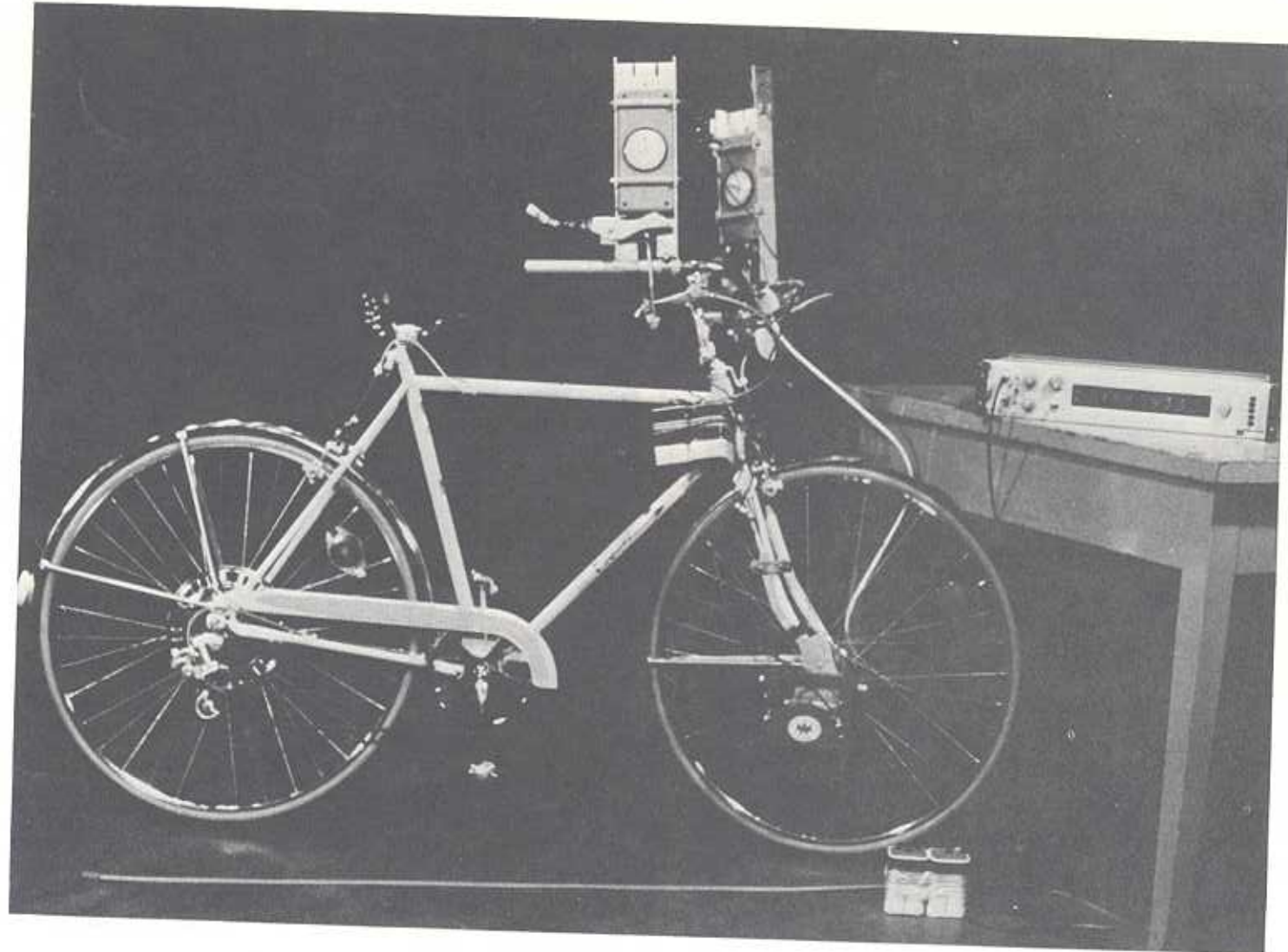
Figure 19. Bicycle Brake Performance Test Equipment-Installed
