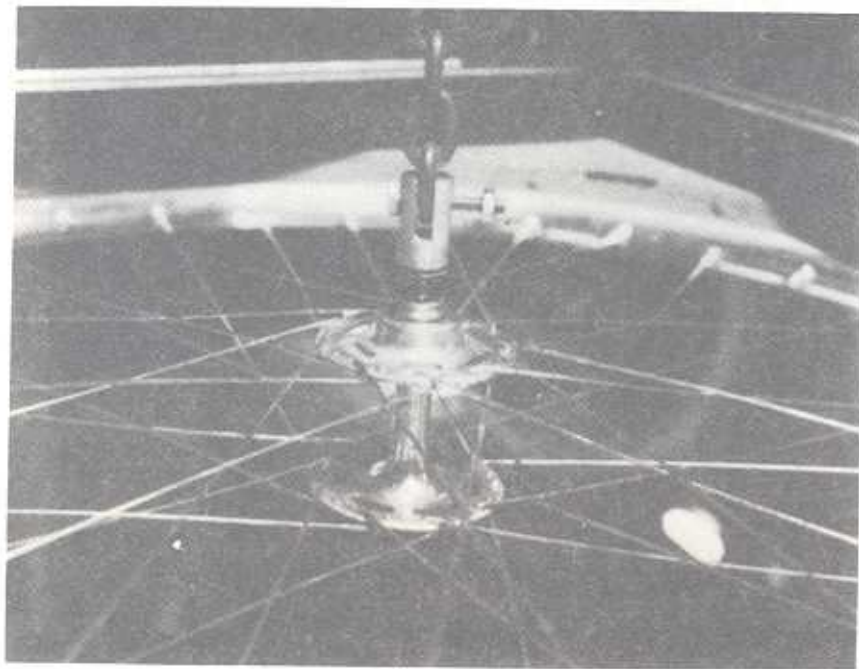
Figure 34. Rim Test Fixture-Axle Coupling Detail
