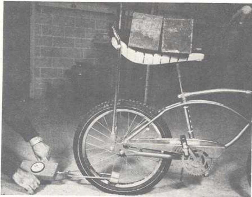
Figure 8. Test Setup for Measurement of Coefficient of Friction
