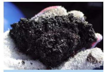
A sample of oil sand consisting of sand, water and bitumen. (Photo by Melina Mara/The Washington Post, reproduced with permission.)
