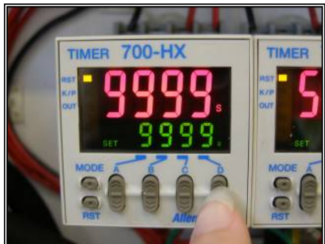
Figure 46. Step 5 Timer set to maximum time
