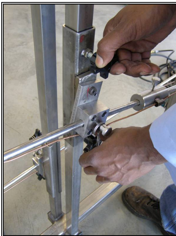
Figure 17. Step 13 Adjust top burner height.
