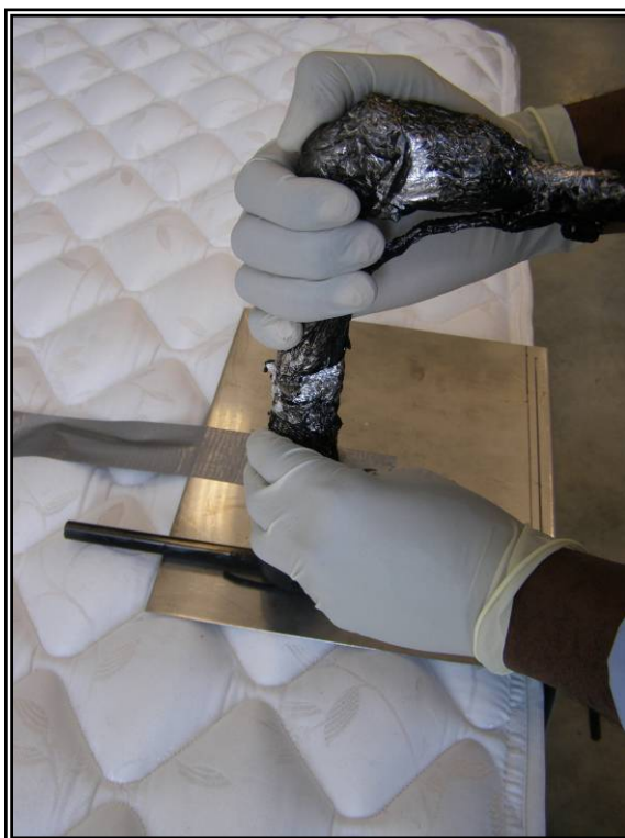
Figure 18. Step 14 Make burner face parallel to platen.
