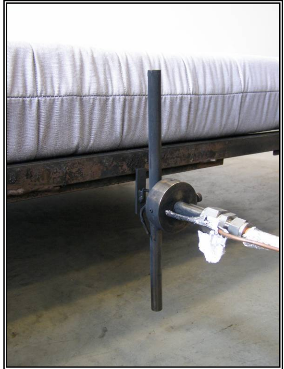
Figure 35. 16.1 Alignment of the side burner for thin specimens.
