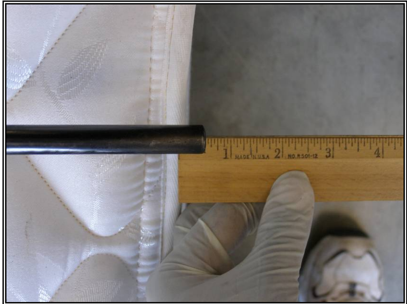
Figure 29. Step 26 Final placement of top burner.
