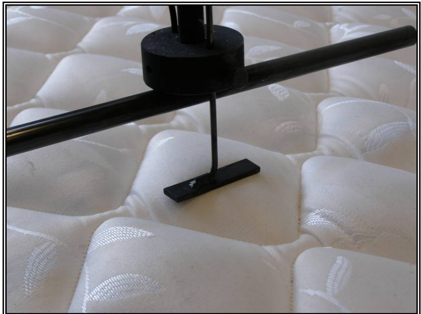
Figure 28. Step 25 Burner stand-off foot should not be in a depression.
