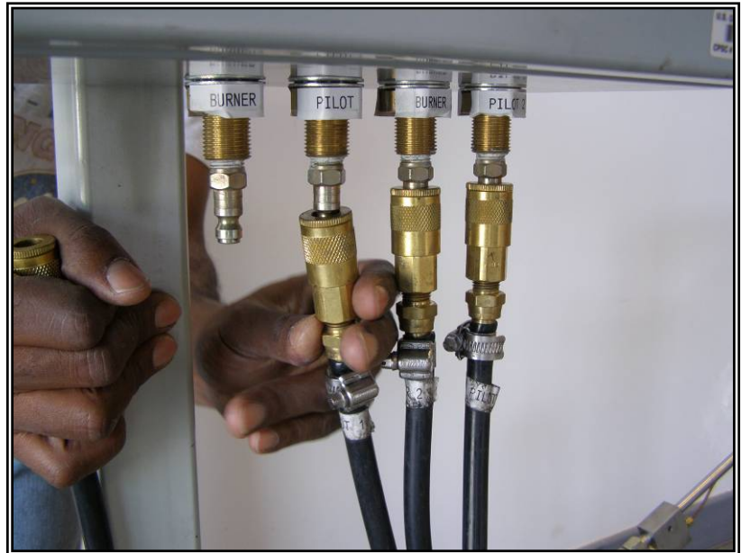
Figure 10. Step 3 Connect hoses to control box.
