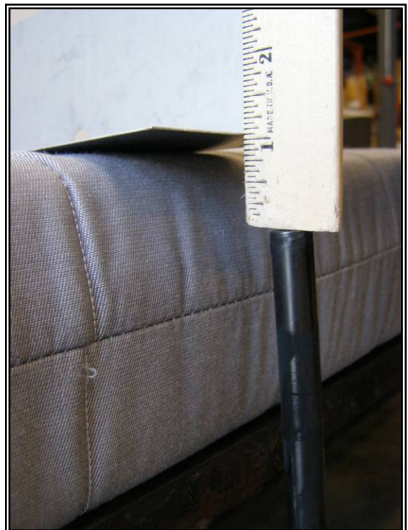
Figure 36. 16.1 Side burner one inch below top of specimen.
