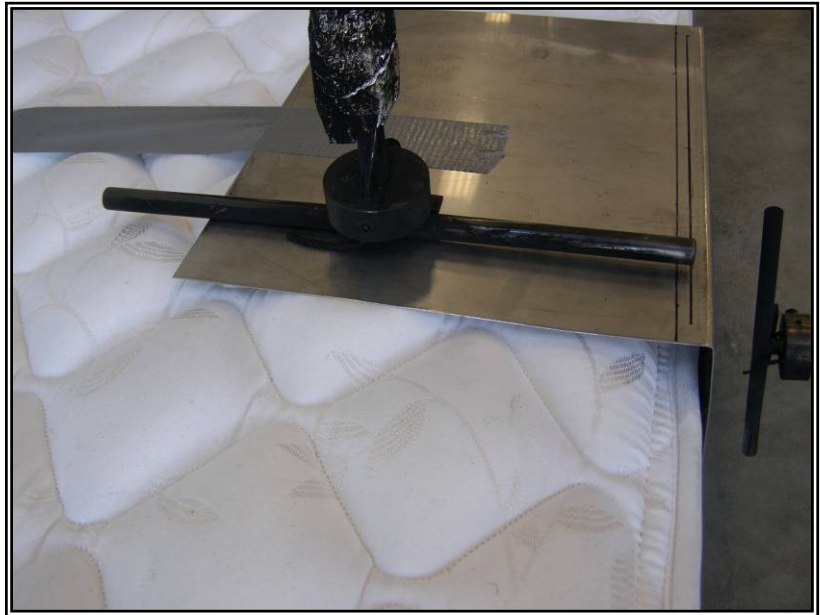
Figure 19. Step 15 Position burner head.
