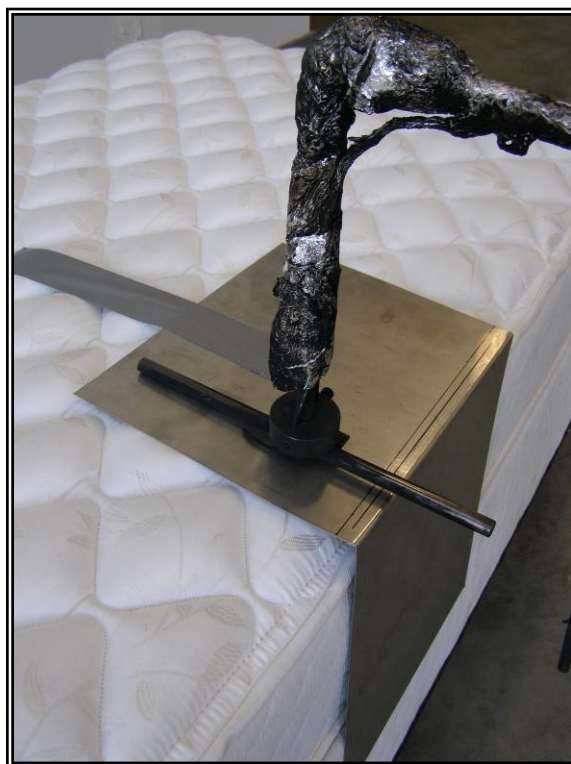
Figure 16. Step 12 Lower the top burner onto the platen.
