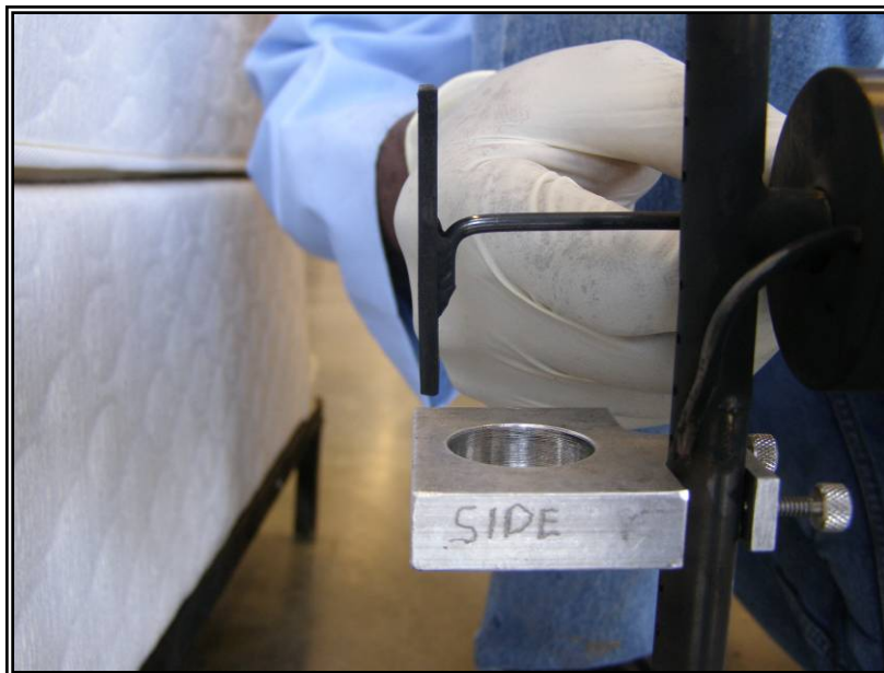
Figure 25. Step 21 Set stand-off foot distance with jig.
