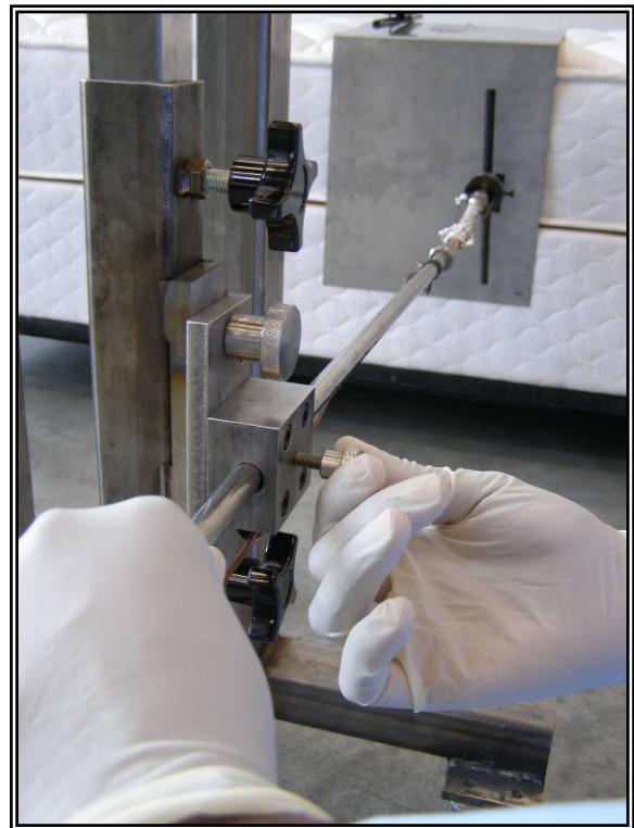
Figure 20. Step 16 Position the side burner.
