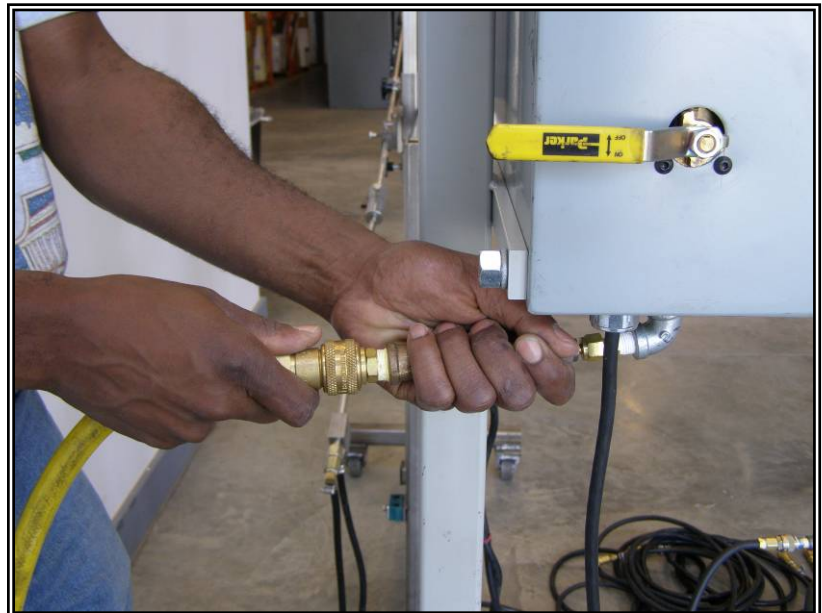
Figure 9. Step 2 Connect propane supply.
