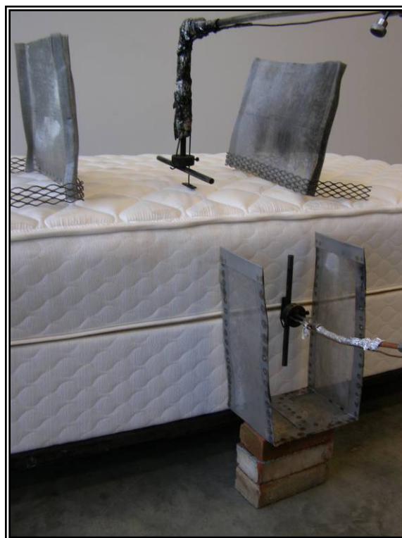
Figure 32. Step 35 Screens placed around burners.
