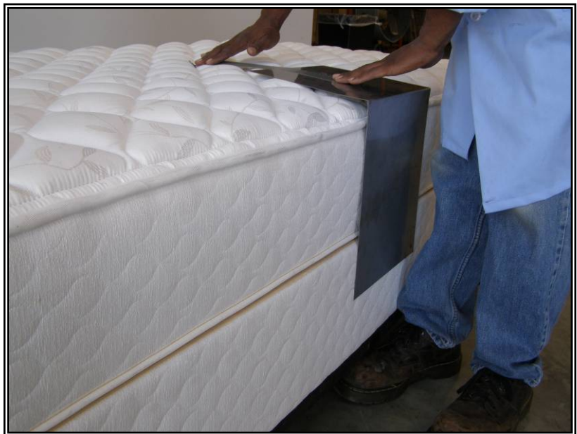
Figure 14. Step 10 Secure the platen.
