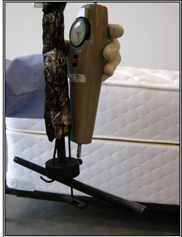
Figure 27. Step 23 Measure downward force using spring scale.
