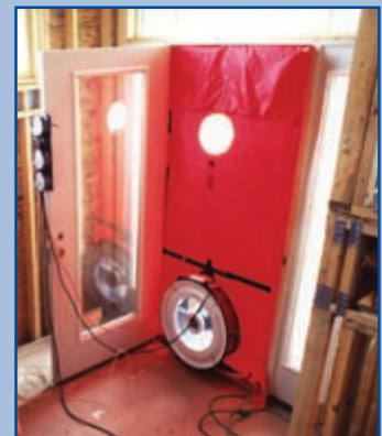
Home airtightness is tested using a blower door.
