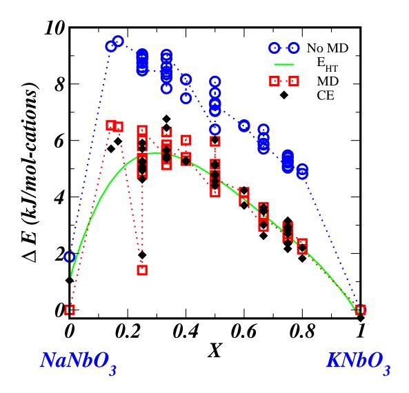
FIG. 1: Comparison of VASP formation energies, $\Delta E_f$ , that were calculated by convensional 0 K relaxations ( $\bigcirc$ , "No MD") with  $\Delta E_f$  from 0 K relaxations that followed 300 K annealing runs ( $\square$ , "MD"). Filled diamonds ( $\blacklozenge$ ) indicate the cluster-expansion fit to the annealed set, and the solid curve is the high temperature cluster expansion limit for the total energy.
