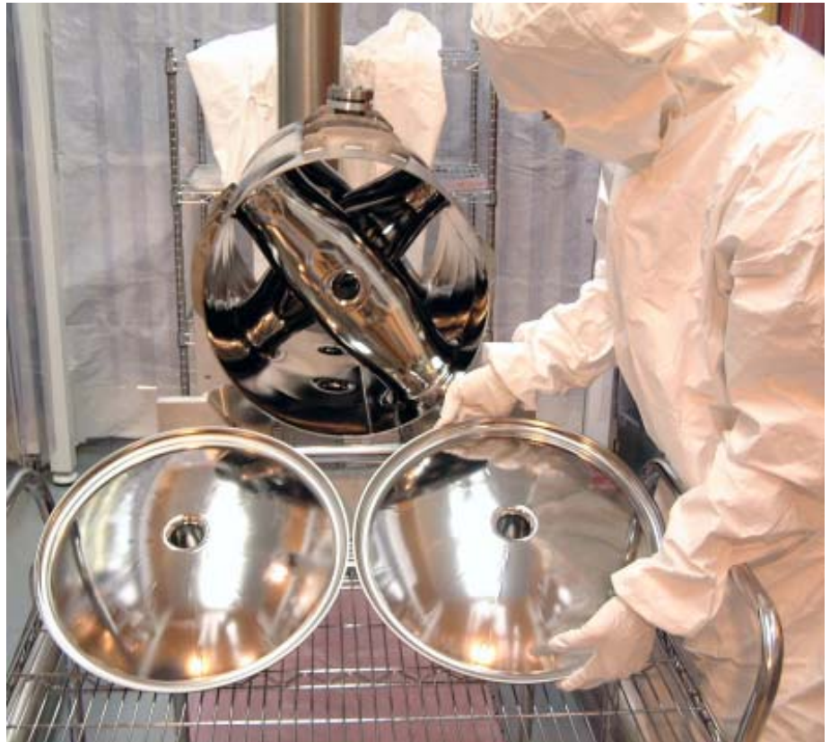
A superconducting triple-spoke cavity is prepared for electropolishing in a clean room. The cavities will lead to significant improvements in the performance of superconducting niobium cavities and could translate into a potential savings in the cost of a heavy-ion linear accelerator, such as that required for the proposed Facility for Rare Isotope Beams.
