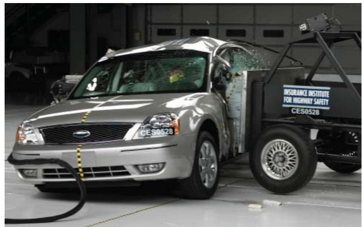
This undated photo provided by the Insurance Institute for Highway Safety shows a side impact test on a 2006 Ford Five Hundred vehicle with optional side airbags. (AP Photo/ Insurance Institute for Highway Safety)
