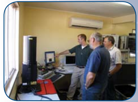
A representative from Sigma Space Corporation trains ACRF operations staff in Darwin, Australia, on various components of the new MPL. The lidar, shown at left, will be placed in one of the outdoor instrument shelters, below a hole in the roof for the laser to pulse through.
