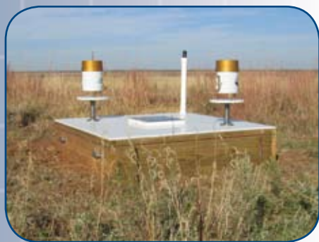
Sets of rain and stream gauges like this one are providing information about water level and flow rates from sites throughout the Whitewater River watershed during the HydroKansas field campaign.
