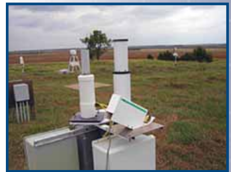
The cylindrical 1-channel (left) and 2-channel (right) NFOV radiometers are collocated with the infrared thermometer (front) at the SGP site.
