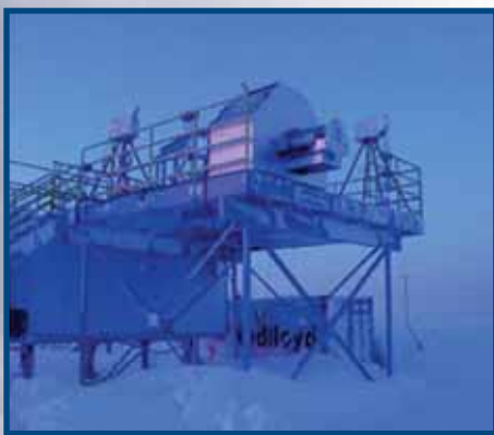
Some of the instruments collecting data during the Arctic Winter Water Vapor IOP included ARM’s microwave radiometer profiler (left) and microwave radiometer (right), and NOAA’s ground-based scanning radiometer (middle).
