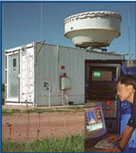
Inside the instrument shelter, the MMCR data system collects radar spectral data and processes these into reflectivity, vertical velocities, and spectral width.
