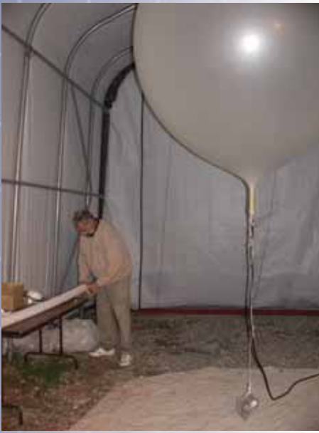
During the experiment, 56 balloons carrying 112 radiosonde packages were launched; typically, multiple packages were launched on the same balloon for comparison purposes.
