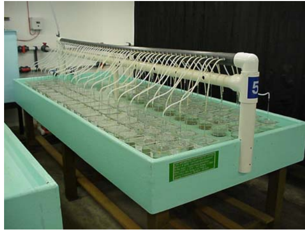
Figure 14.1. Sediment toxicity test system.
