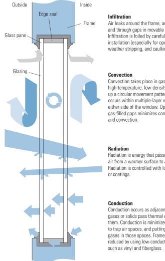
Air leaks around the frame, around the sash, and through gaps in movable window parts. Infiltration is foiled by careful design and installation (especially for operable windows), weather stripping, and caulking.
