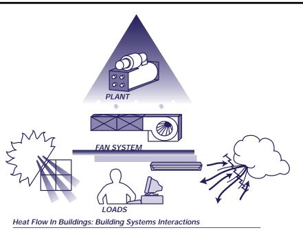
Figure 2 shows the interaction of heating, cooling, and electrical loads with the HVAC equipment. Arrows indicate heat flow pathways. Reducing heating, cooling, and electrical loads reduces the demand on HVAC equipment, thus saving energy.
