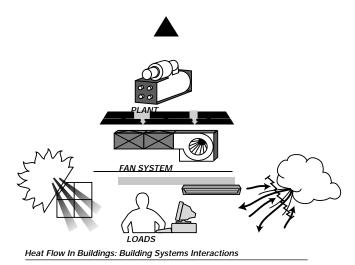
Figure 2 shows the interaction of heating, cooling, and electrical loads with the HVAC equipment. Arrows indicate heat flow pathways. Reducing heating, cooling, and electrical loads reduces the demand on HVAC equipment, thus saving energy.
