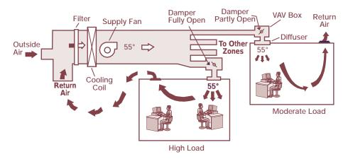
In a VAV system, dampers control the flow of chilled air to respond to changes in cooling load.
