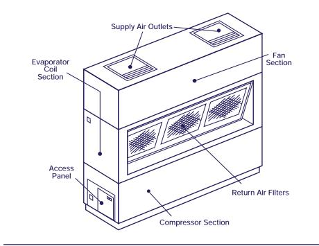
Figure 10: Split-System Packaged Units
