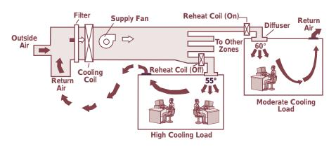
In this example, the room with the moderate cooling load is reheating its air from  $55^{\circ}$  to  $60^{\circ}$  F.
