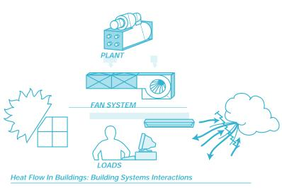
Figure 2 shows the interaction of heating, cooling, and electrical loads with the HVAC equipment. Arrows indicate heat flow pathways. Reducing heating, cooling, and electrical loads reduces the demand on HVAC equipment, thus saving energy.
