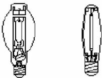
Due to their intensity, HID lighting systems are useful for lighting large areas from high ceilings, and range from 50 to 2,000 watts each. Older HID installations are often mercury vapor lamps, an extremely inefficient design. Like fluorescent lamps, HID systems have ballasts, and systems built before 1978 may contain potentially harmful substances such as PCBs (Polychlorinated biphenyls).
