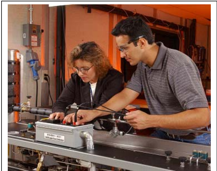
Fig. 1. A dual rotor turbine meter is installed in the test section of the 2 L Hydrocarbon Liquid Flow Standard.
