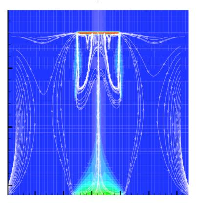
Left: Density-driven vortex made the fluid with higher  $CO_2$  concentration "snap-off" from the source—the supercritical  $CO_2$  plume.
