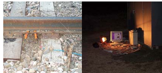
Figure 5. Field test setup of piezoelectric device (orange clamps held device during glue up)
