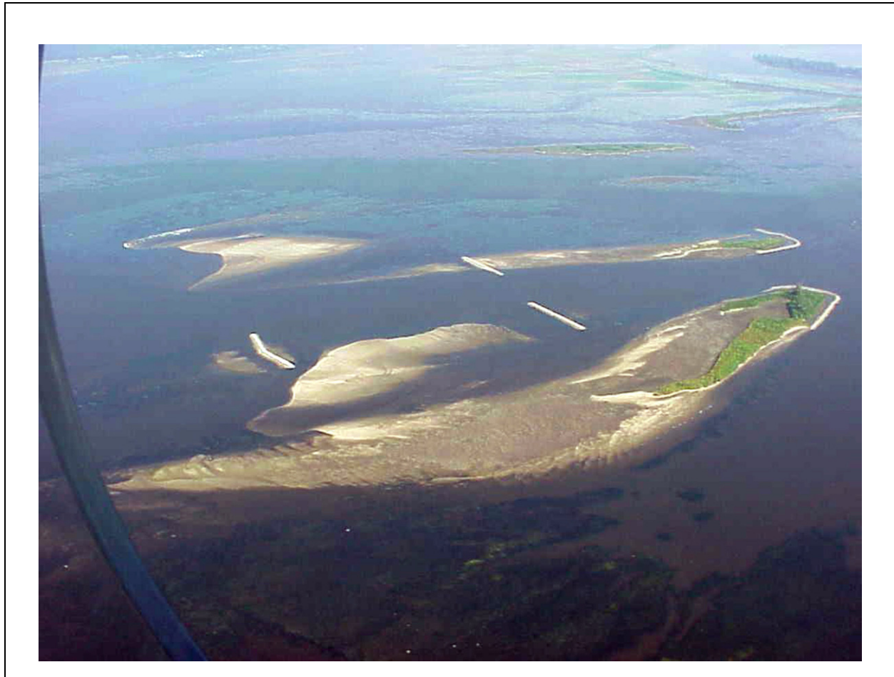
Figure 30: Seed Islands Constructed and “Growing” on Upper Mississippi River NW&FR
