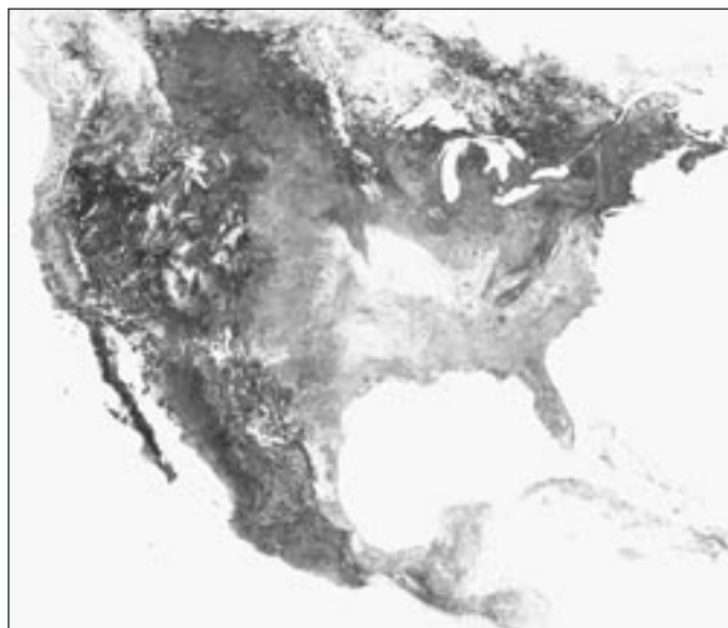
Bihemispherical Albedo (White-Sky Albedo) for North America for the period April 22 - May 7, 2000, calculated from the MODIS BRDF/Albedo product algorithm using data from the Terra MODIS near-infrared channel (Band 2). In this image, cloud cover has obscured some regions in the central U.S. as well as other smaller areas shown in white. Light tones in the southeastern U.S. indicate strong reflectance from leaf cover, while much of the more northern regions remains leafless.
