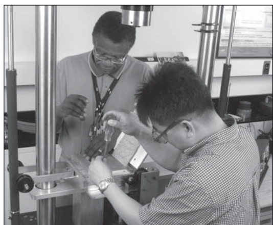
Mechanical Folding Device attached to MTS testing platform being loaded with a piece of woven ballistic fabric.
