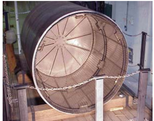
Argonne's new multiport dryer technology for the forest industry could greatly improve the efficiency of dryers used in paper mills. The photo shows a fully assembled Multiport dryer insert installed in Kadant Johnson half-dryer.
