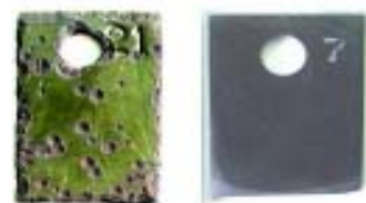
Alloy 600 ANL alloy New alloy developed to resist metal dusting (right), a long-standing corrosion problem for materials used in the chemical and petrochemical industries (left).
