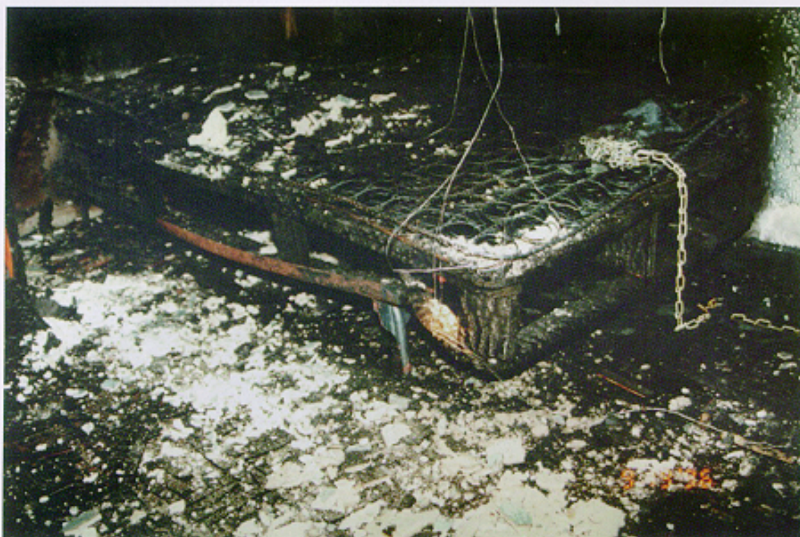
FIGURE 54. Photograph of the bed showing bed frame deformation. Experiment 3.
