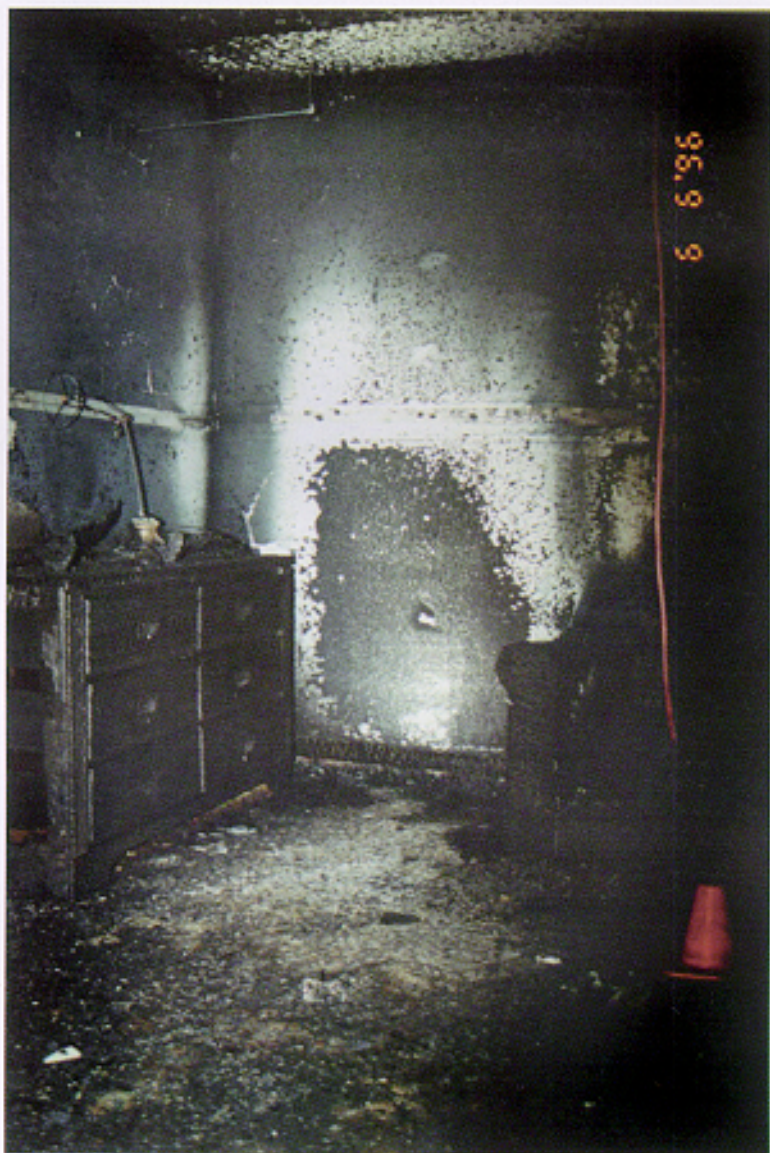
FIGURE 31. Photograph of the clean burn on the wall between the chair and the dresser. Experiment 2.
