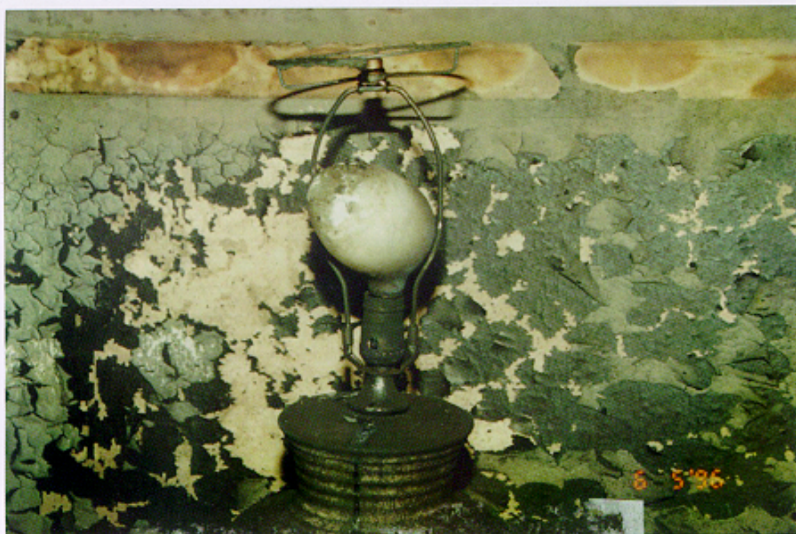
FIGURE 43. Photograph of a deformed light bulb located in the lamp on the nightstand. Experiment 1.
