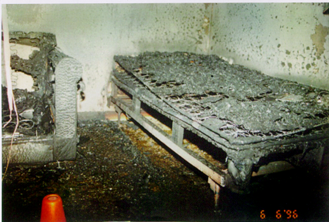
FIGURE 39. Photograph of the condition of the bed and the protected floor area below. Experiment 2.
