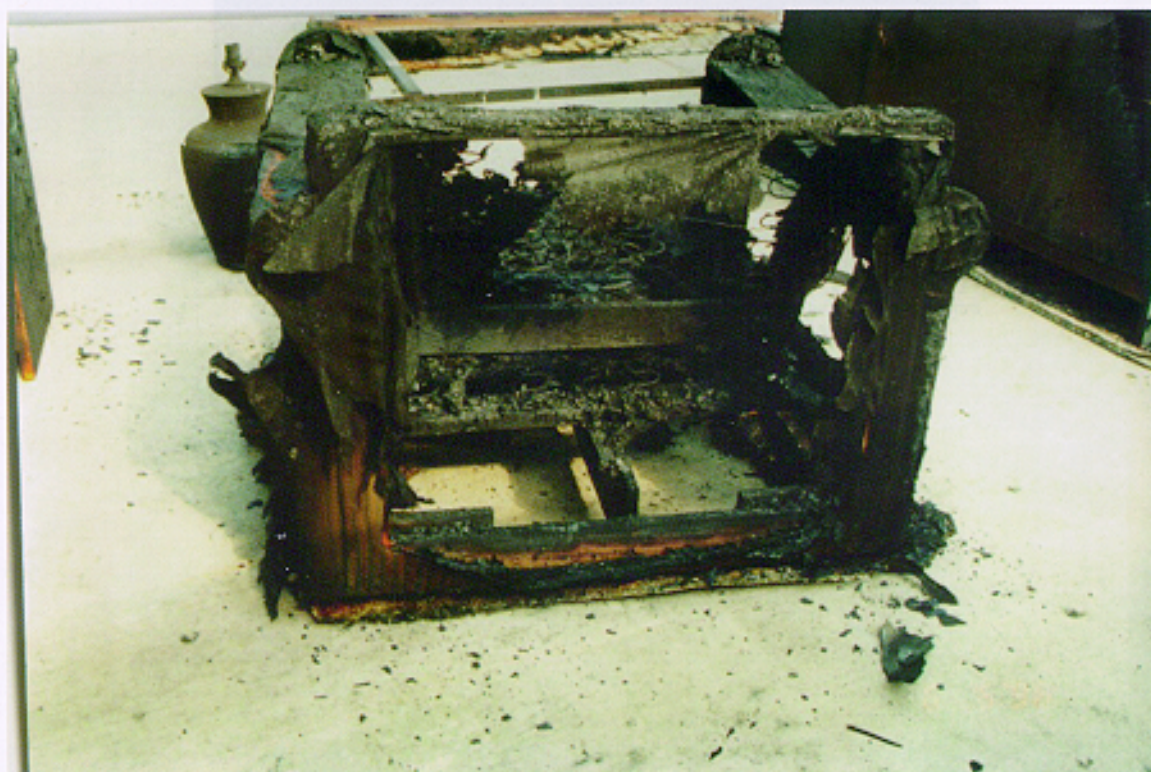
FIGURE 37. Photograph of the rear surface of the chair, located against the wall. Experiment 1.
