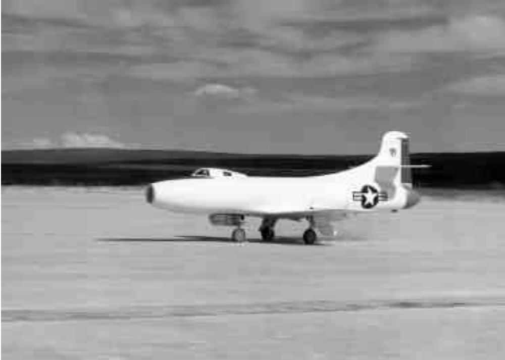
The D-558-I on the lakebed at the High-Speed Flight Research Station. Crossfield made the first of his fourteen D-558-I flights on November 27, 1950, and flew the last on June 10, 1953. The Skystreak was the workhorse of early transonic research, due to its ability to cruise at speeds close to Mach 1 for prolonged periods. (E-226)
