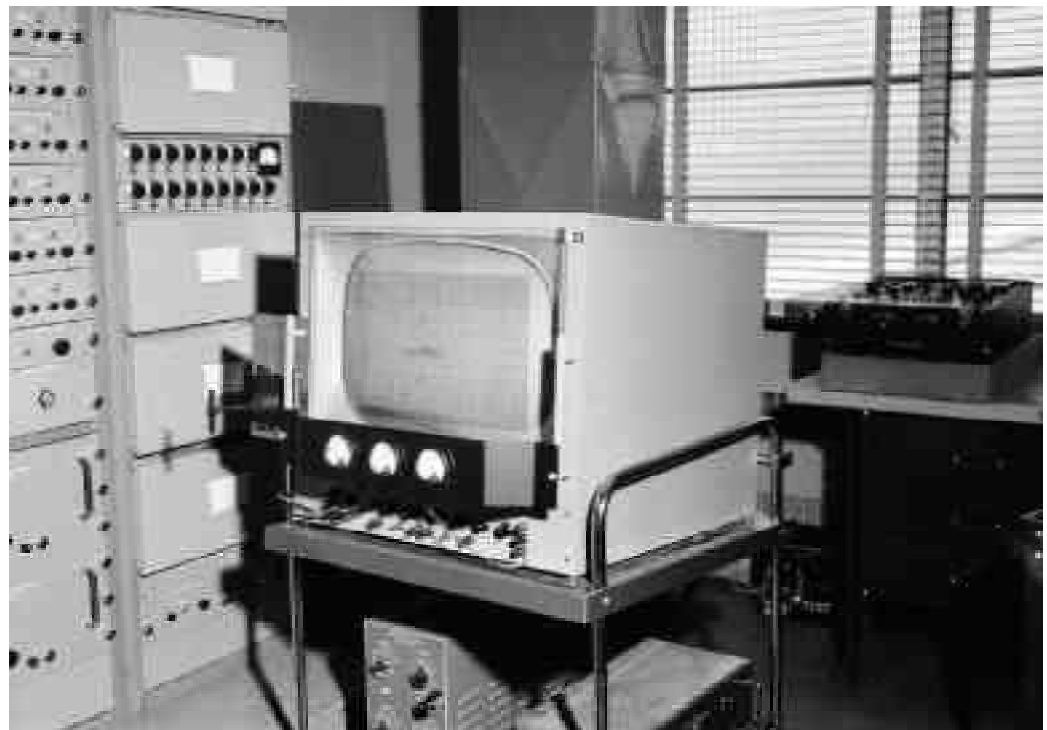
An early analog computer used to predict aircraft stability and control behavior. This machine represented a major breakthrough, as it enabled the research pilot to gain experience on the ground, and gave advance warning of dangerous flight conditions. Day recalled later that the computer predictions of the X-2's behavior at Mach 3 exactly matched the actual flight characteristics from Apt's flight. (E57-2946)
