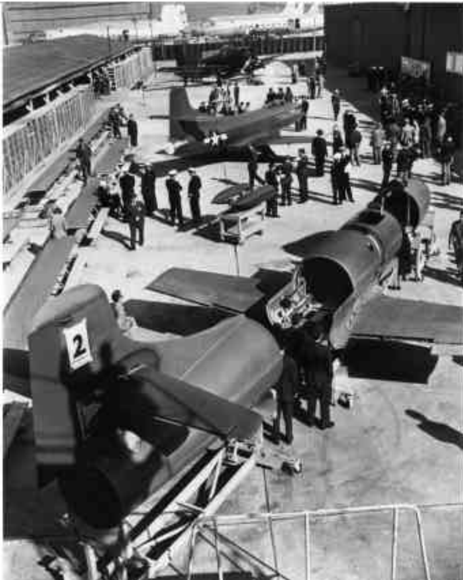
The D-558-1 Skystreak under construction (photograph provided by Tony Landis).
