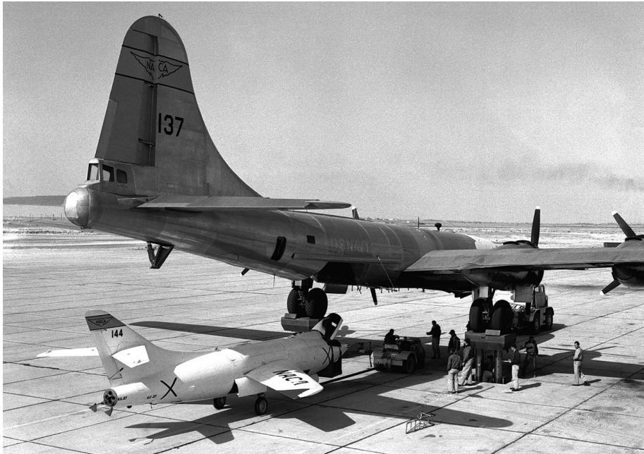
D-558-2 number two being positioned under its Navy P2B mothership being elevated on hydraulic jacks. When the Skyrocket was in position, the P2B would be lowered so the D-558-2 could be attached to the bomb bay of the "mothership" for climb to altitude before being launched. (NASA photo E-1013).
