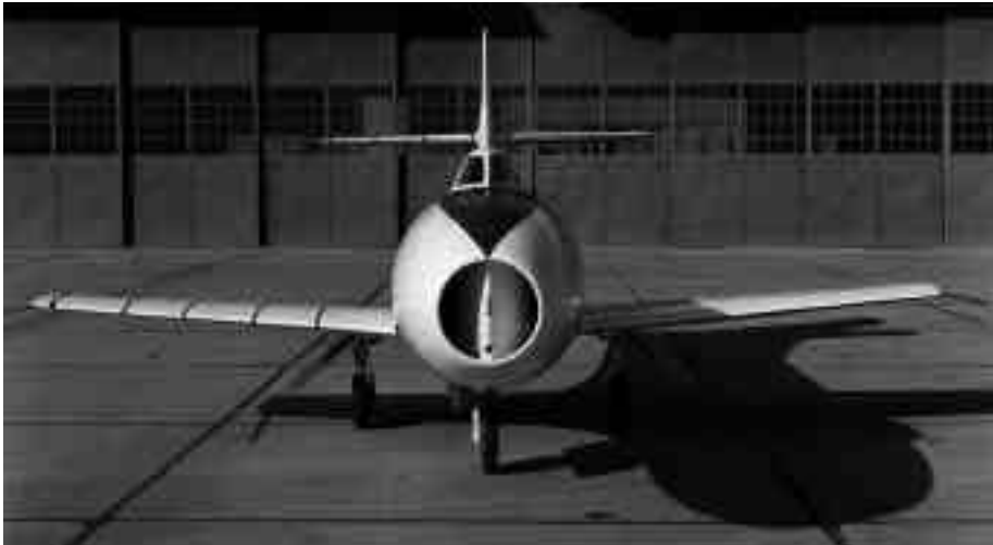
Head-on view of the D-558-1 showing the bifurcation in the engine inlet, forcing the intake air to go on either side of the pilot. (NASA photo E49-89).
