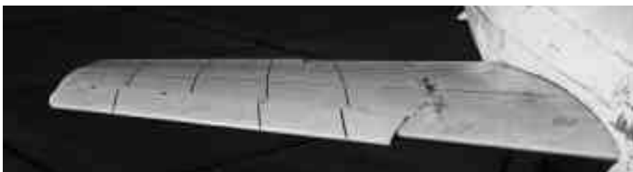
Wing slat on a D-558-2. (NASA photo E-816).
