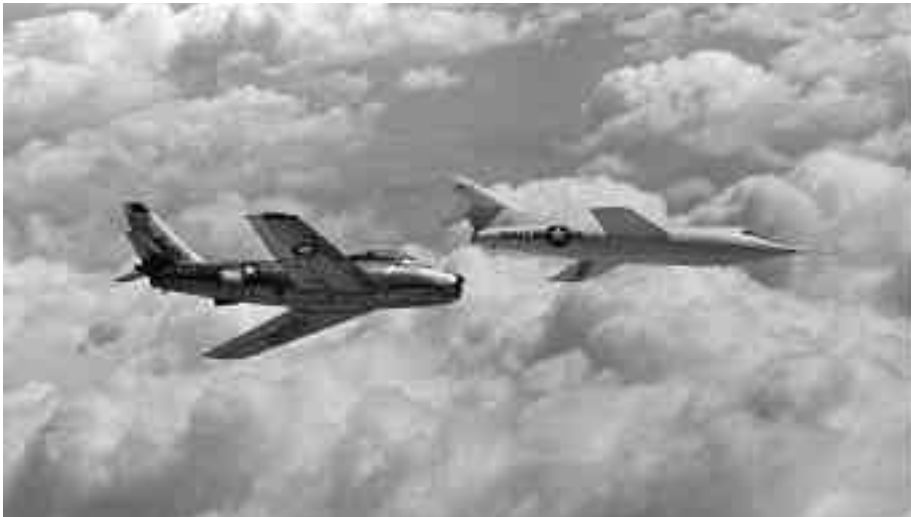
D-558-2 number two returning from a research flight with an F-86 flying behind it as a chase aircraft. (NASA photo E-3996).
