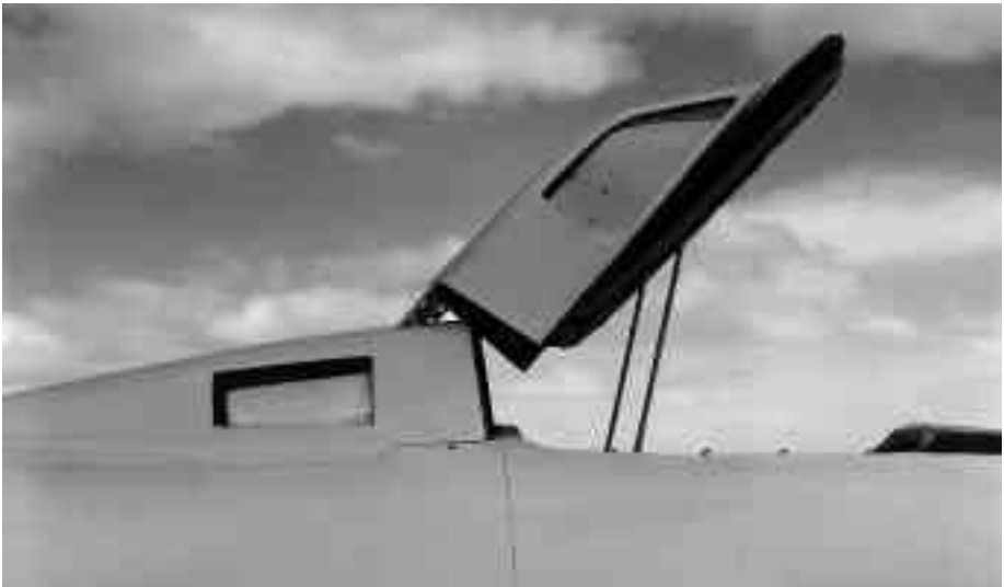
The cockpit of the D-558-1 showing how it opened. (NASA photo E49-86).
