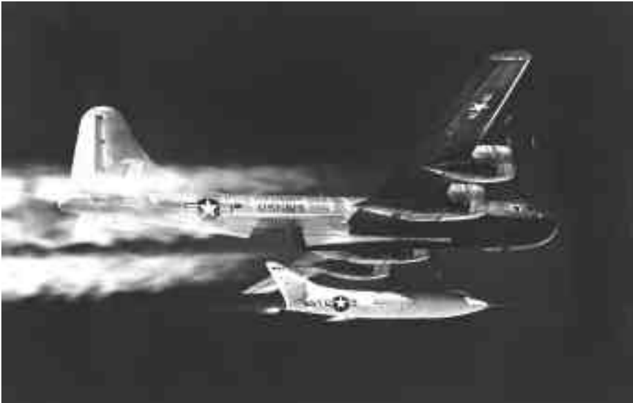
Number two D-558-2 Skyrocket being launched from a Navy P2B mothership. (NASA photo E-2478).
