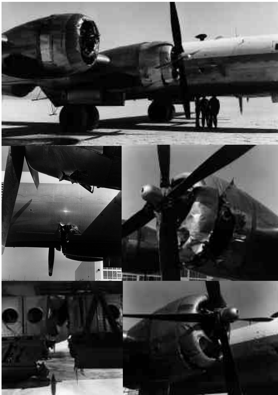
Series of photos showing damage to the P2B March 22, 1956, when the number four engine exploded and shed its propeller. (NASA photos E-2200, E-2203, E-2210, E-2213, E-2221) .
