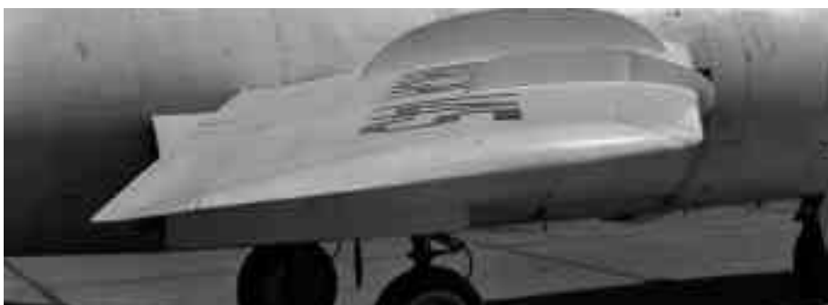
Wing fences on a D-558-2. (NASA photo E-580).
