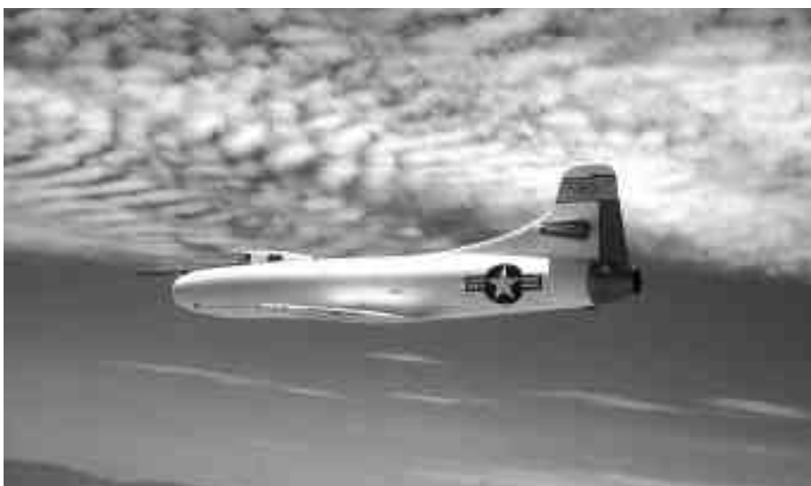
D-558-1 in flight on one of its transonic research missions. (NASA photo E-713).
