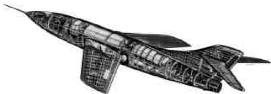
Cutaway view of the D-588-2. (Photo provided by Tony Landis).
