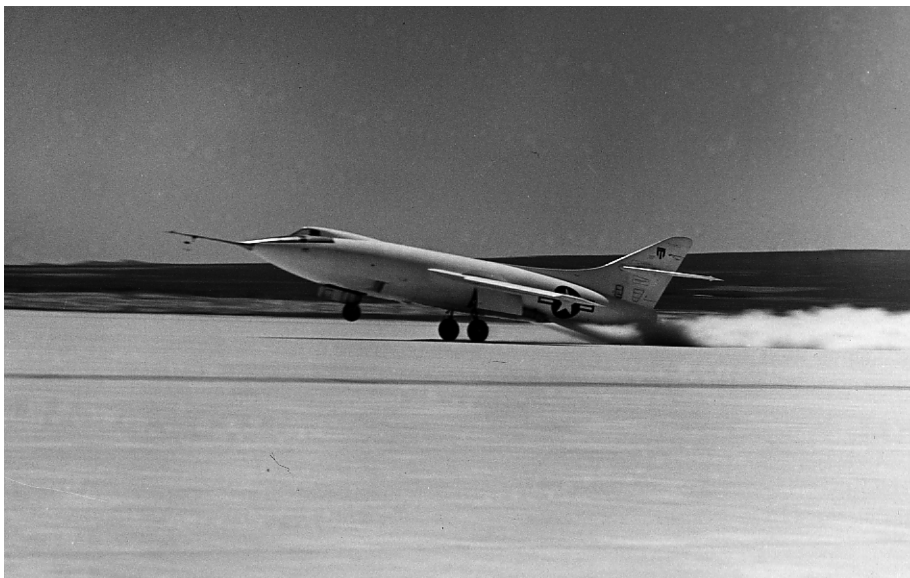
D-558-2 taking off with jet assisted take-off (JATO). (NASA photo E49-219).
