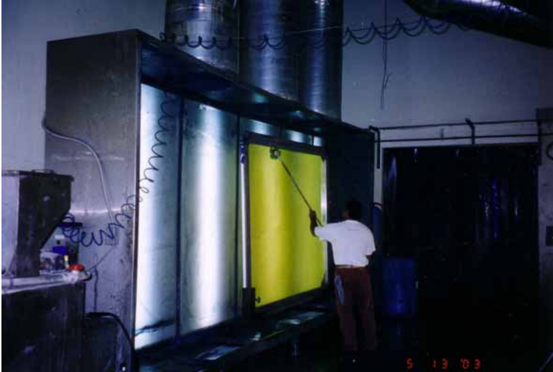
Figure 4-2. Screen and Cleaning System at Southern California Screen Printing.
