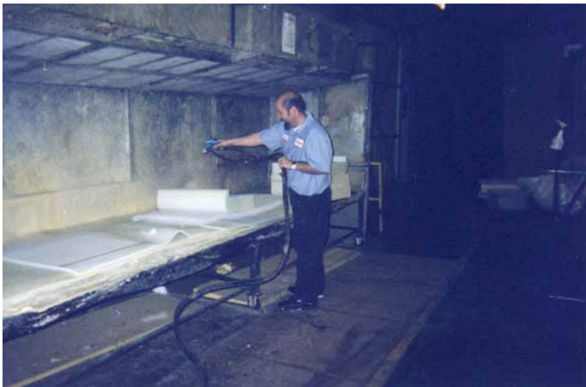
Figure 3-8. Adhesive Spray Booth at Hickory Springs.
