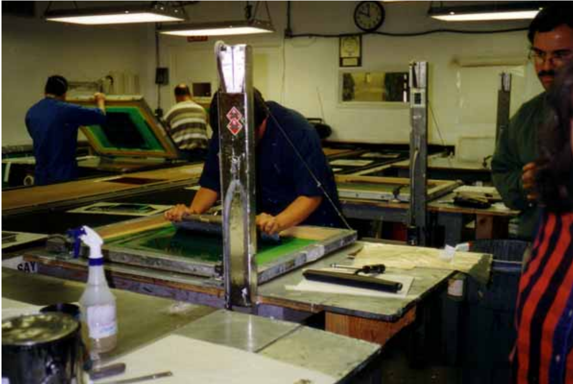
Figure 4-3. Screen Printing at Nelson Nameplate.
