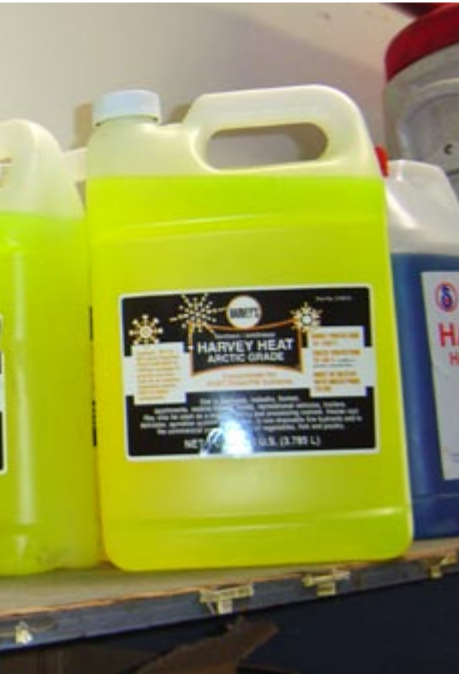
Propylene glycol is a non-toxic heat transfer fluid that provides freeze protection.
