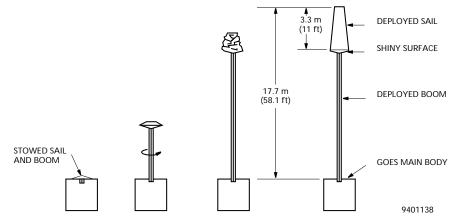
Two redundant, miniature, dc-torque motors control the extension rate of the boom. When the boom is completely deployed, a redundant pair of switches on each motor actuate, disconnecting motor power which stops the motors. If any pair of switches fails to operate, the motor continues to run as long as the execute signal is being sent. If this happens, the end of the lanyard will disconnect from its reel to prevent damage.
