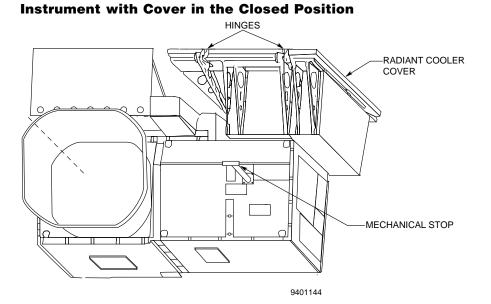
Microswitches on the deployment hinges indicate stowed and fully deployed positions. Deployment is also indicated by changes in temperature of the lower cooler housing, the radiator, and the infrared detector.
