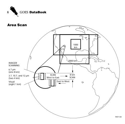
A priority scan feature allows improved scheduling of small area and mesoscale scans for short range forecasts and storm warnings. Imager large area scans of 3000 by 3000 kilometers (1864 by 1864 statute miles) are accomplished in three minutes and small area scans of 1000 by 1000 kilometers (621 by 621 statute miles) can be made in 41 seconds. A 3000- by 3000-kilometer area can be sounded in 43 minutes, and full earth can be imaged in 26 minutes.
