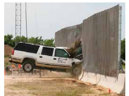
SANDIA conducted crash tests to determine viability of different types of fences.
