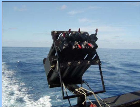
Autolauncher installed on the Horizon Hawaii
