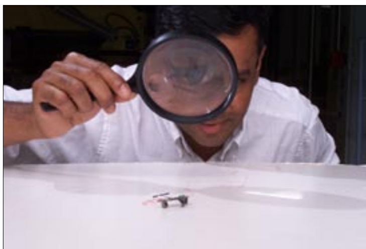
Venu Varma of ORNL is shown with a micro-robot, a battery-powered sensor that can travel under doors, for example, and detect chemical and biological agents.
