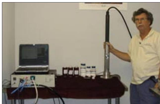
John Schindler, Vice President of R&D for Austin AI, stands with the CP-1000 XRF cone penetrometer in a lab stand configuration.
