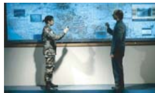
Air Force engineers demonstrate the AFRL/IF Datawall, a self-contained and ultra high-resolution large screen display with multi-modal, wireless interaction that allows users to display and manipulate multiple applications through a collaborative environment.
