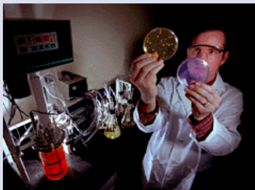
SNL researcher Mark Tucker examines two petri dishes: one with a simulant of anthrax growing in it, the other treated with the decontaminating foam developed at SNL. The nonhazardous foam begins neutralizing both chemical and biological agents in minutes.
